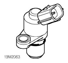
The camshaft position sensor has two functions. The first is to enable the ECM to run a sequential fuelling mode. The second is to measure the actual cam period, this measurement is achieved using teeth on the camshafts to indicate when the valve opens and closes.
