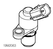
The CMP sensor on VVC engines is located on the rear face of the cylinder head and reads off a reluctor on the inlet camshaft.
