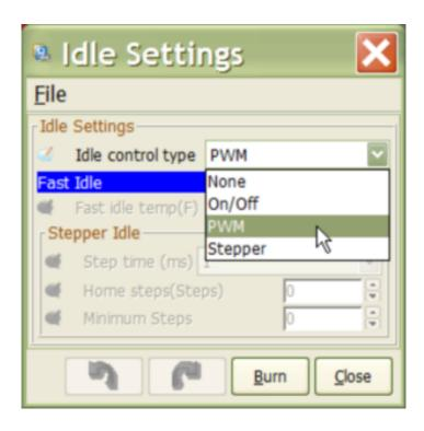
The temperature-versus-DC is selected under the Idle - PWM Duty Cycle selection. Note the relationship between temperature and PWM DC can be altered by simply moving the blue dots in the curve, or by selecting the table for manual entry as shown here:
