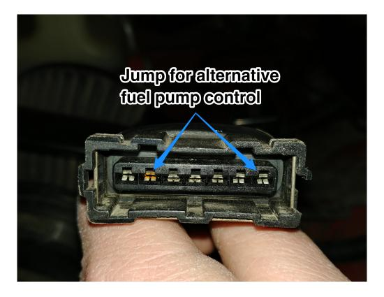
Once the above jumper is in place, the fuel pump pin in TunerStudio should be set to A9.
